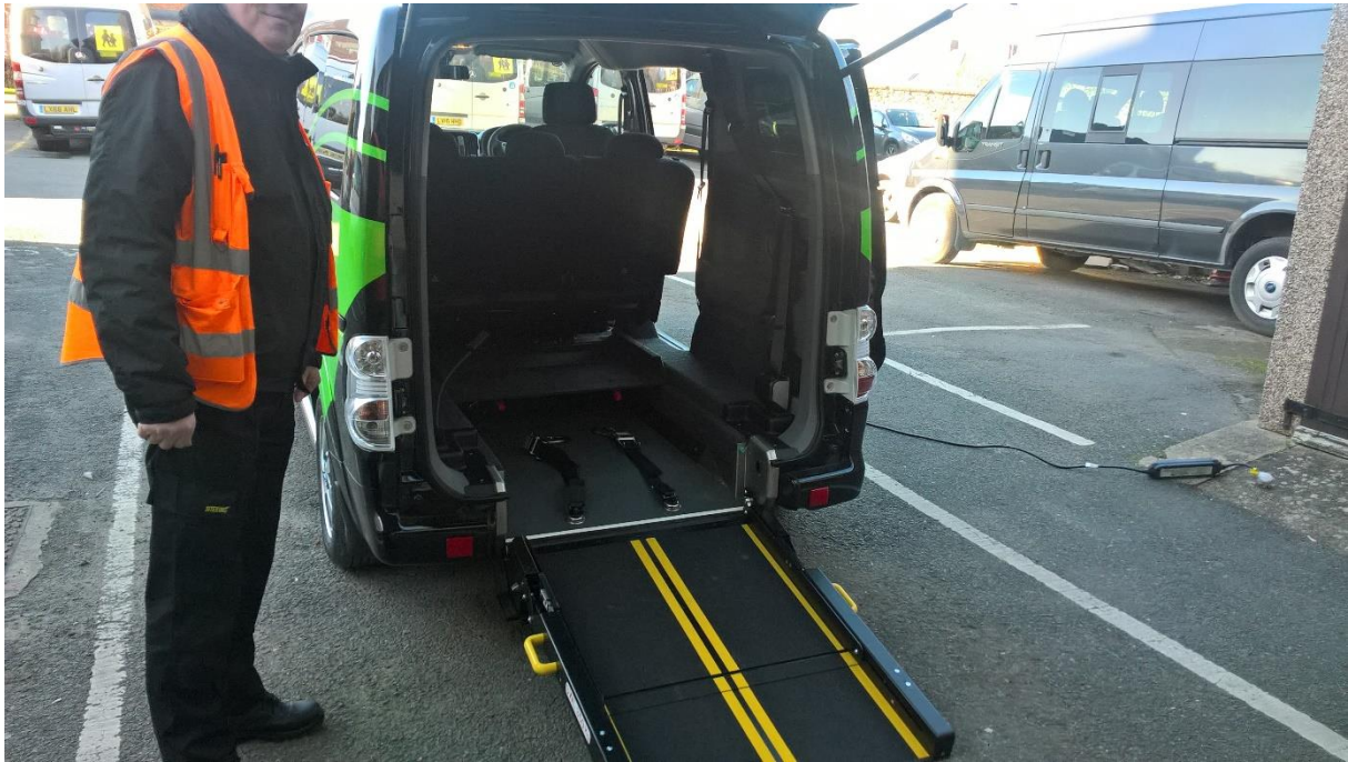
Trail of an accessible Nissan eNV200 by OCC's Integrated Transport Unit
