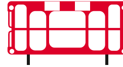
Typical traffic barrier with tapping rail
